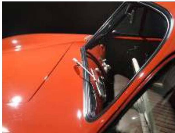
The first 356s were split window with two panes of glass. In 1953 a single windshield with a crease in the center was installed.
