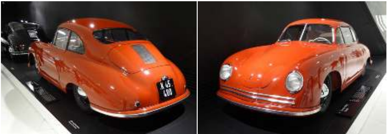
This is the 356/2 coupe built in 1948. It had a 1,086 cc 40 HP motor with a top speed 140 km/hr (87 mph). This is one of the 52 first Gmünd Austria hand built cars. The engine was moved behind the axle to provide a space for two small jump seats and a luggage compartment. It too was made from aluminum.
