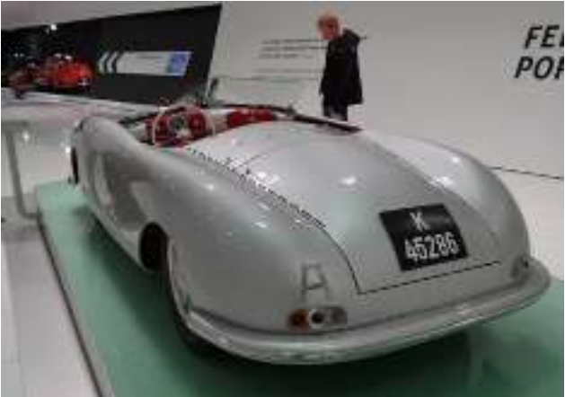
There can be only one Number One, and this is it. It is the 356 type 1. It was hand built from aluminum in the spring of 1948. It featured a mid-engine 35 hp. VW motor.
