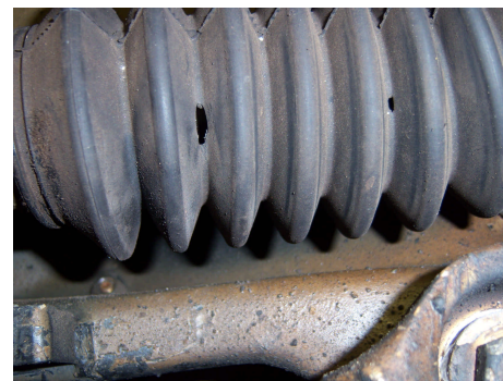
Figure 8: Steering Rack Boot (Bad)
