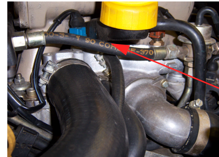
Figure 34: Front Fuel Line
