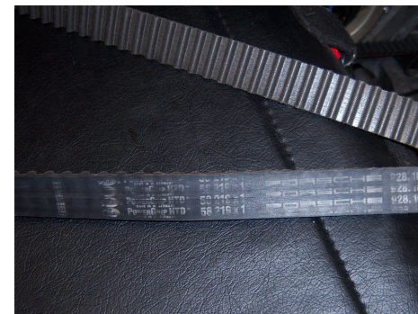
Figure 46: 44k-mile 19 year-old factory-installed timing belt
