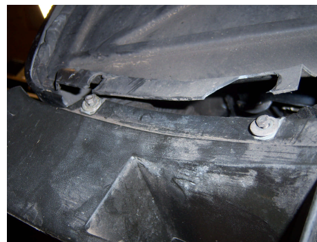
Figure 13: Busted Splash Guards from Bottoming Out
