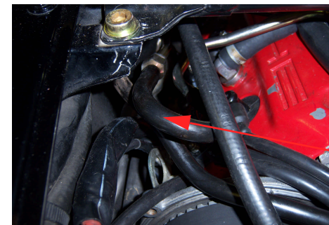
Figure 36: Front Fuel Line
