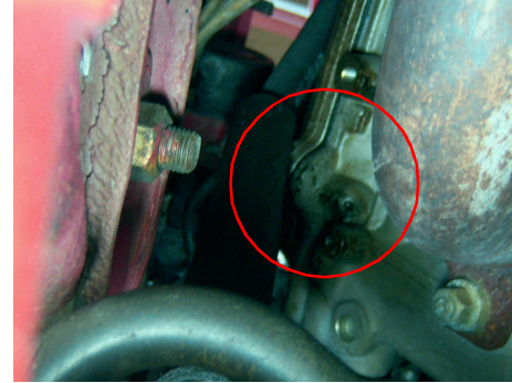
Figure 20: Leaking Cam Cover
